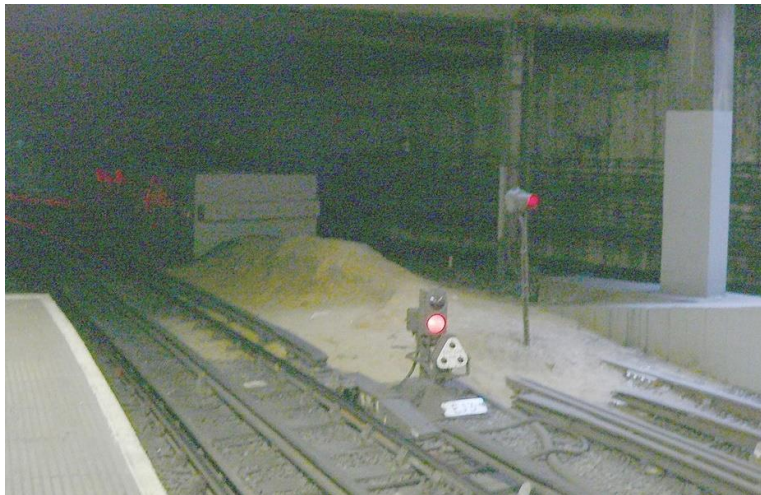
Figure 6: London Underground Mounded Sand Drag
