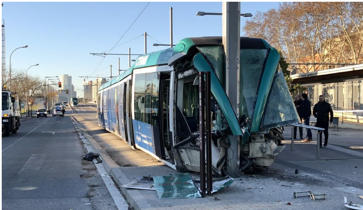
Figure 1: Tram crash in Barcelona, January 2019, showing the fatal consequences of a relatively low speed front-end collision with a traction pole
