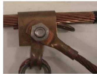
**Compression (Crimped) Sleeve**
